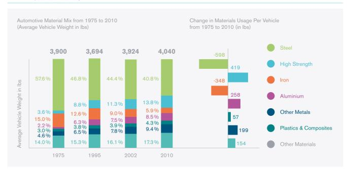
Today, lightweighting is a crucial factor leading to the rapid expansion of the global automotive composite market. Different lightweight materials have always been part of the automotive materials mix, but as shown in Fig 12, **high strength steel, aluminium and**
